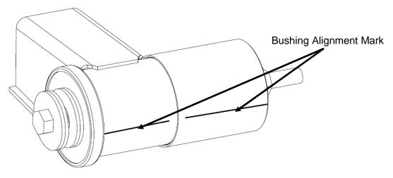
Figure 6 Bushing Alignment Marks
