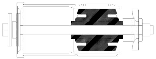
Figure 3 (Bushing in Arm sleeve before removal)
