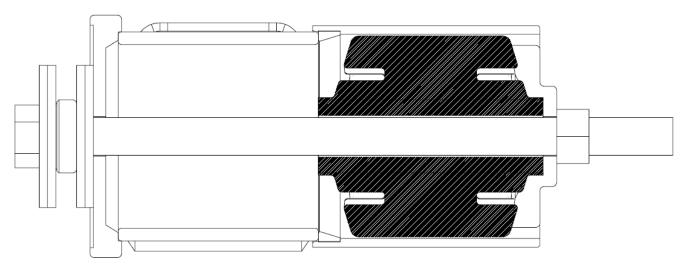
Figure 5 Bushing in Transition Tube before installation
